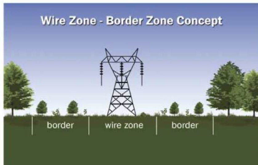
Figure 1: Wire Zone – Border Zone Concept: This diagram is provided for informational purposes only and is not drawn to scale or intended for use as a specification detail.
